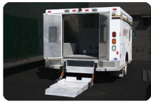
Prison Transport Lifts 750 lbs. weight capacity
